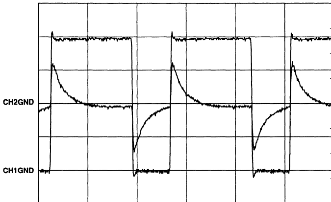
FIGURE 3. CH1 IS THE VARIABLE DUTY CYCLE INPUT VOLTAGE (VS) CH2 IS THE VOLTAGE AT L- AND R+ INPUTS OF THE HIP2030
